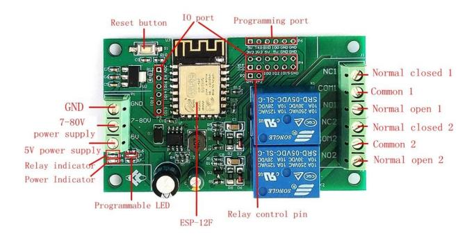
Programming port: ESP8266's GND, RX, TX, 5V are respectively connected to the GND, TX, RX, 5V of the external TTL serial port module. IO0 needs to be connected to GND when downloading, and then disconnect the connection between IO0 and GND after the download is complete;
