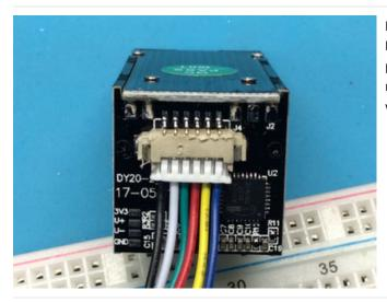
If your sensor has different wires, The first wire from the left should be the black wire ground, then the two data pins, RX is the white wire, TX is the green wire then the red power wire. You'll have to cut, strip and solder the wires.
