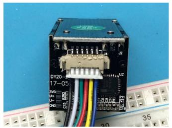
If your sensor has different wires, The first wire from the left should be the black wire ground, then the two data pins, RX is the white wire, TX is the green wire then the red power wire. You'll have to cut, strip and solder the wires.
